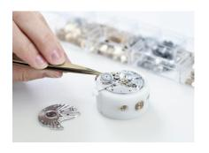
7. Lambda is powered by DUW 1001; the first caliber to bear the name Deutsche Uhrenwerke NOMOS Glashütte—large and slender, with twin mainspring barrels. 29 jewels within ensure flawless functioning, with six of them in hand-polished screwed chatons. Just as they have been for the past 175 years.
